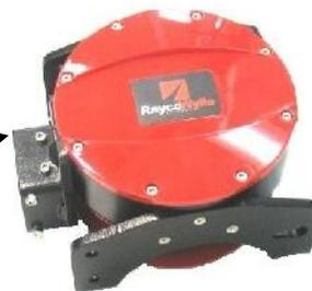
The R140 provides an audio and visual alarm when the hook reaches the maximum safe height to the boom tip. The display is wired to the tip mounted ATB switch with a cable on a lattice boom or a cable reeling drum on a telescopic boom. A second switch, weight and jib cable, if necessary, can be added to monitor both the main and auxiliary hoist on the same display. The display has an internal relay that can be integrated with a function lock out system. (sold separately)
