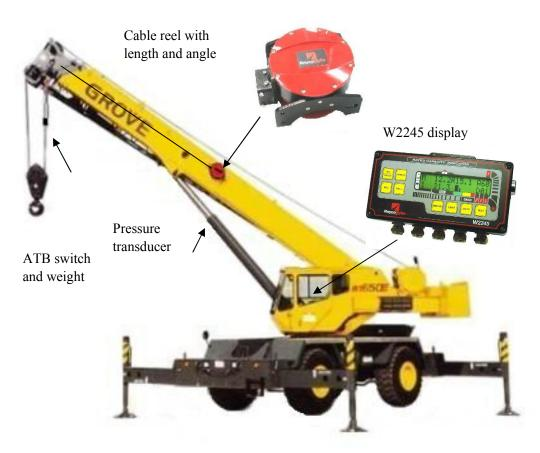
This is the most popular configuration for the W2245 system. For telescopic boom cranes with 360 degree load charts this is the most cost effective LMI system on the market. This is a true Load Moment Indicator (LMI) because it actually measures the load on the boom from the pressure sensors mounted on the lift cylinder. This style of system is accurate, reliable, low maintenance, and easy to use. \*\*\* Only for use on cranes with 360 degree capacity charts \*\*\*
