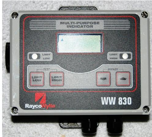
The Wylie Boom Angle Indicator puts accurate boom position information where a crane operator needs it – in the operator's cab. The high and low angle warning feature is very helpful when operating a crane under power lines or when carrying out repetitive operations.
