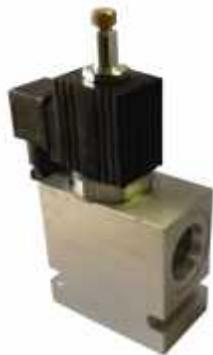
40 GPM valve with two #16 SAE ports. This valve is used for 3/4" I.D. or smaller lines. Supply voltage is 12V.
